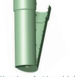
1. Insert large base disc into each half. 2. Clip two halves together
