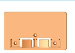
Screw or double sided foam tape to wall - approx. 100mm or 4" from floor.
