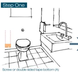
Screw or double sided tape bottom (A) bracket to wall approx. 100mm or 4" from floor. (See overleaf for bracket instructions)
